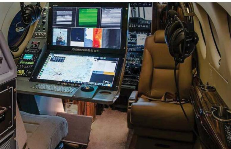
Each operator console has two large 23" multi-touch screens with several new features to facilitate ease of operation and superior situational overview. Sensor data, maps and reports are presented in pre-assigned windows on the screen. Dedicated window layouts or "profiles" are optimised for specific mission types. The operator can at any time switch between the mission types and/or save a personalized configuration to always be ready to meet the current mission objectives.
