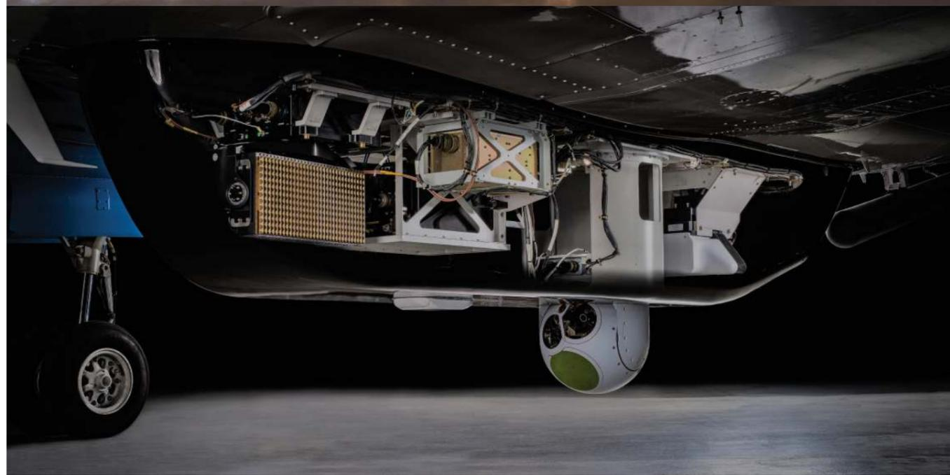
The search radar, EO/IR sensor and IR/UV scanner are housed in a radome under the belly of the aircraft. The EO/IR sensor is mounted on a hoist mechanism for maximum field of view in flight and maximum protection during take off and landing.
