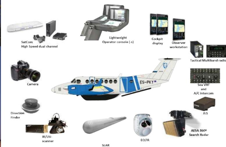
The MSS 7000 for the Estonian Police and Border Guard seamlessly integrates an extensive suite of sensors and communication equipment to make the aircraft an excellent tool for a wide range of surveillance tasks.
