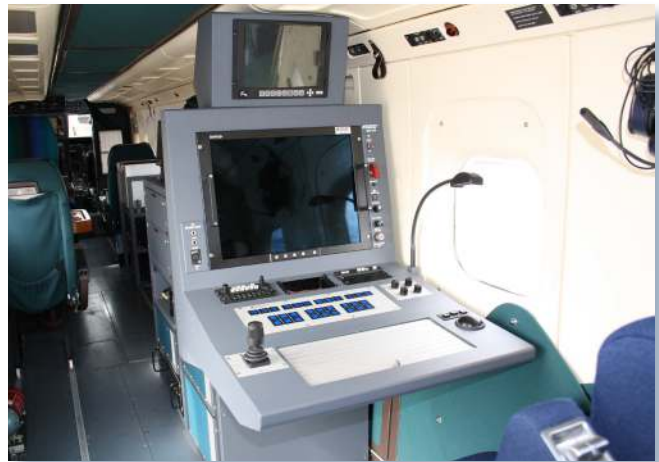
Each of the two MSS 6000 work stations gives the operator full control of the system including all sensors and communication assets.
