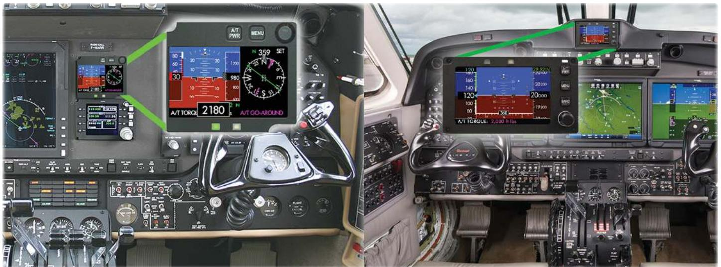
Certified and Available for King Air Pro Line 21 and Pro Line Fusion Flight Decks the ThrustSense® Autothrottle is commanded by the Standby Display Unit that serves as the pilot's interface mode for speed and torque selections, and also serves as a standby EFIS system. The Standby Display Unit houses the computer, which controls the Actuator Assembly which physically moves the throttle.
