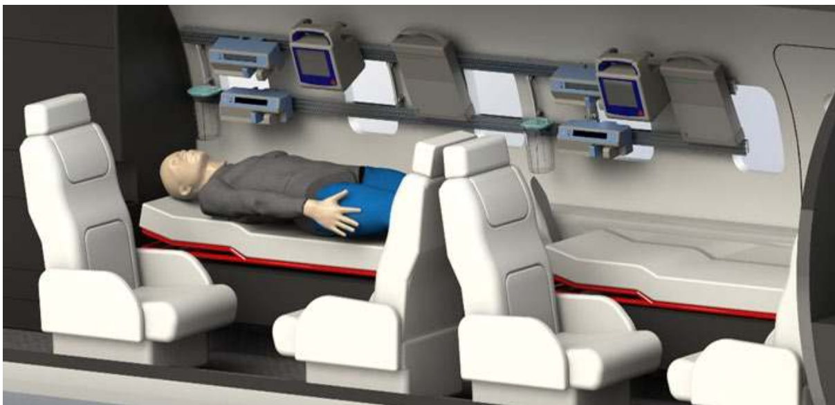
Image: Learjet ambulance aircraft with medical rack.
